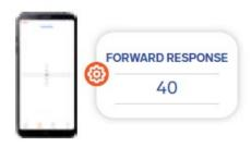
Drive at 40-50km/h and brake firmly. The optimal forward setting is when the tow vehicle and trailer brake as one.
