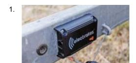
Fasten the unit to the draw bar using the mounting screws provided.
