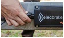
Connect your unit via the Treadway plug and play wiring harness.
